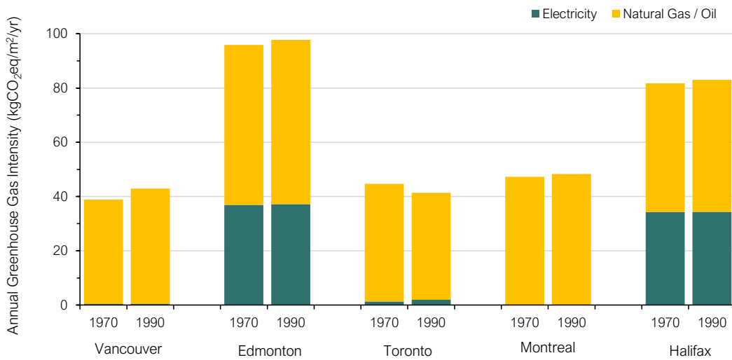
Figure 16. Total greenhouse gas intensity (GHGI) for the 1970s and 1990s mid-rise MURB baseline building archetypes
