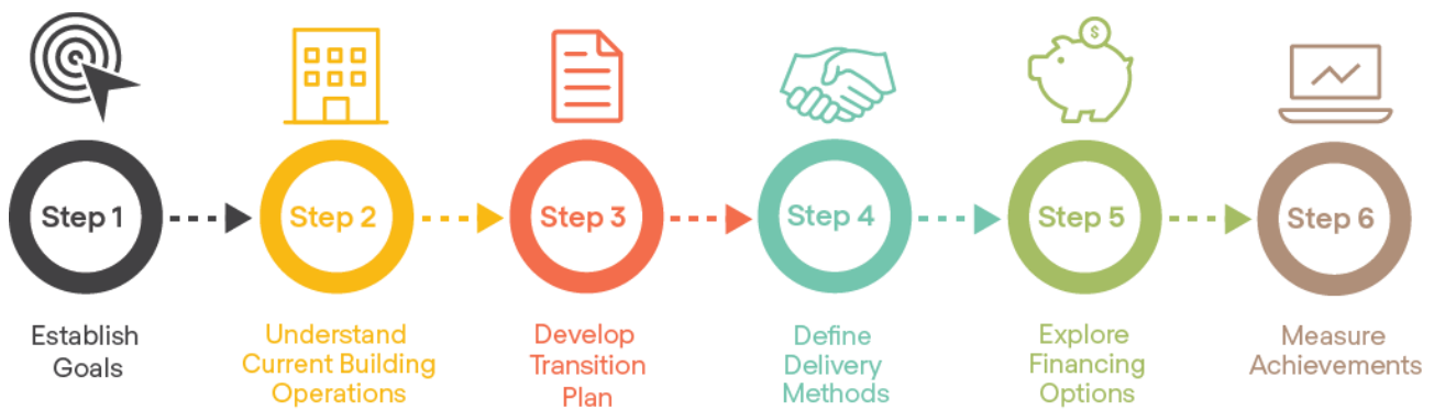
Figure 132. Steps for Achieving Deep Carbon Retrofits
